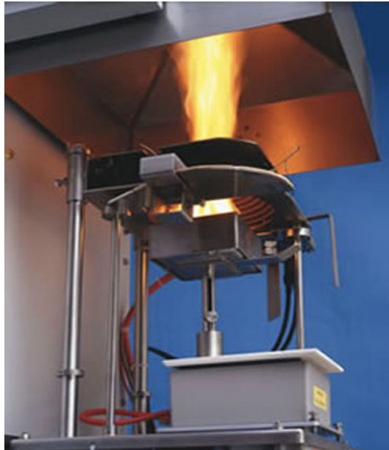
Cone Calorimeter Test: Based on KSF ISO 5660-1 standard
