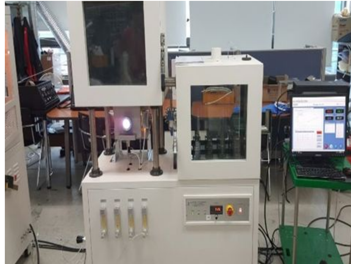
Toxic Gas Emission Test: Based on KSF 2271 standard
